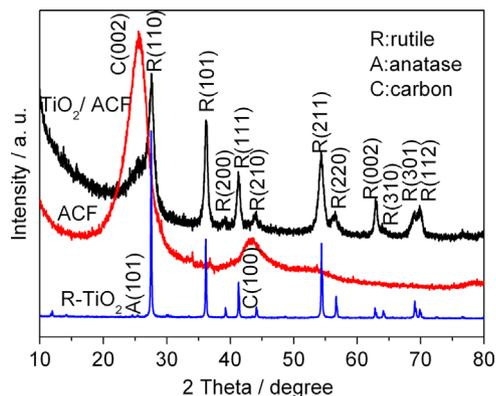
Fig. 1. XRD patterns of  $\text{TiO}_2/\text{ACF}$ , ACF and R- $\text{TiO}_2$ .
