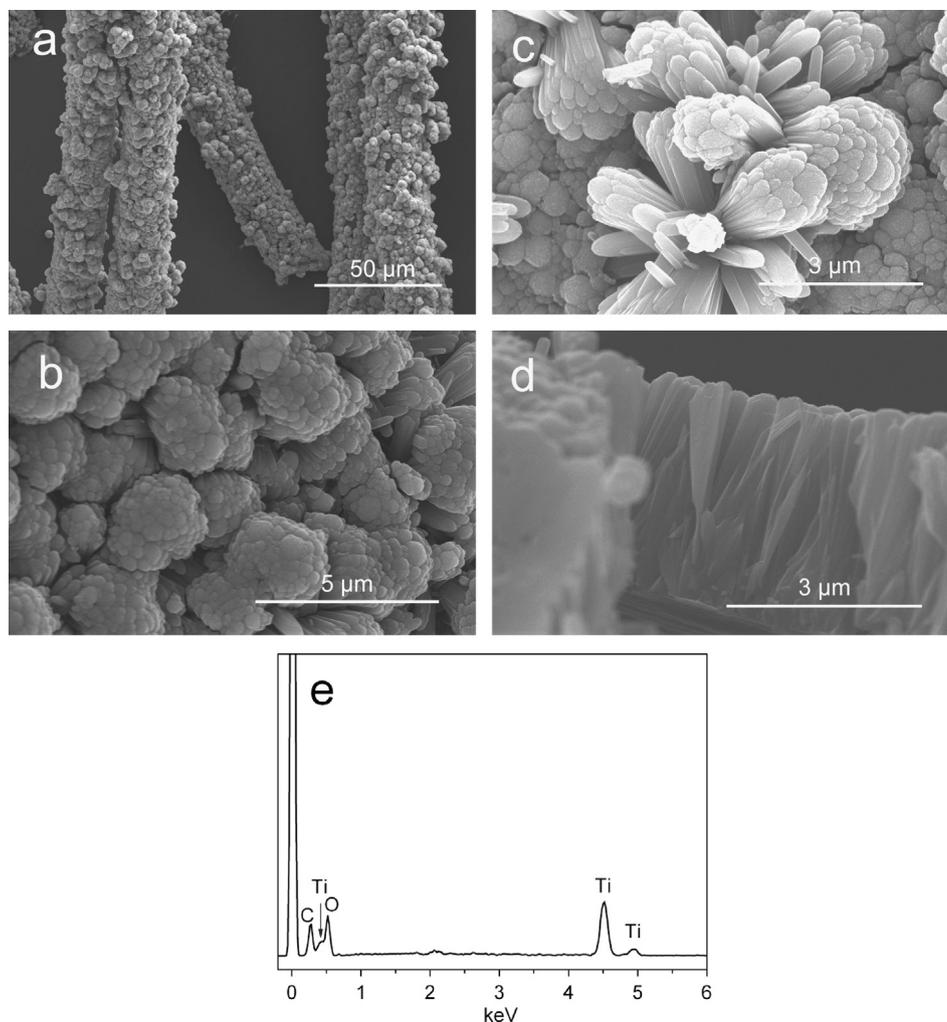
Fig. 2. Low- (a), and high-magnification (b)–(d) SEM images and EDS (e) of  $\text{TiO}_2/\text{ACF}$ .
