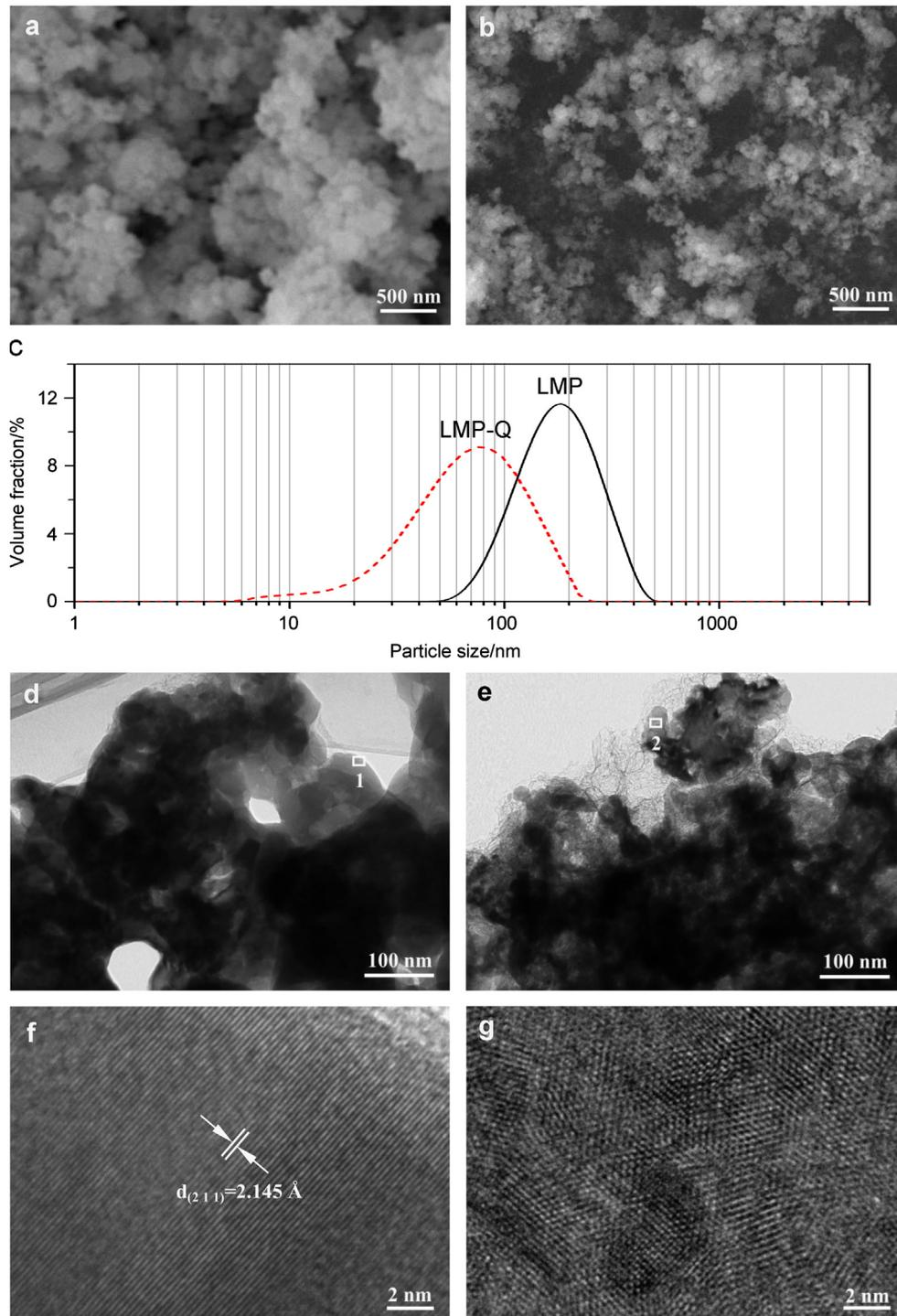
**Fig. 2.** SEM images of LMP (a) and LMP-Q (b), particle size distributions of LMP and LMP-Q (c), TEM images of LMP (d) and LMP-Q (e), HRTEM images of the selected areas 1 (f) and 2 (g).
