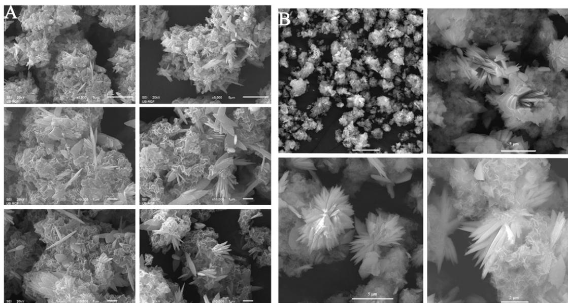
**Fig. 1.** SEM (A), bars: first row 5  $\mu\text{m}$  the other two rows 1  $\mu\text{m}$ ; and FESEM (B), bars: up left 20  $\mu\text{m}$ , up right and down left 5  $\mu\text{m}$ , down right 2  $\mu\text{m}$ ; micrographs of the ZSO structure.
