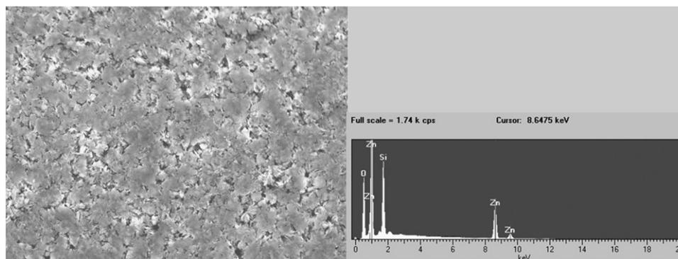
**Fig. 2.** SEM microstructure and EDS analysis of the ZSO powder.
