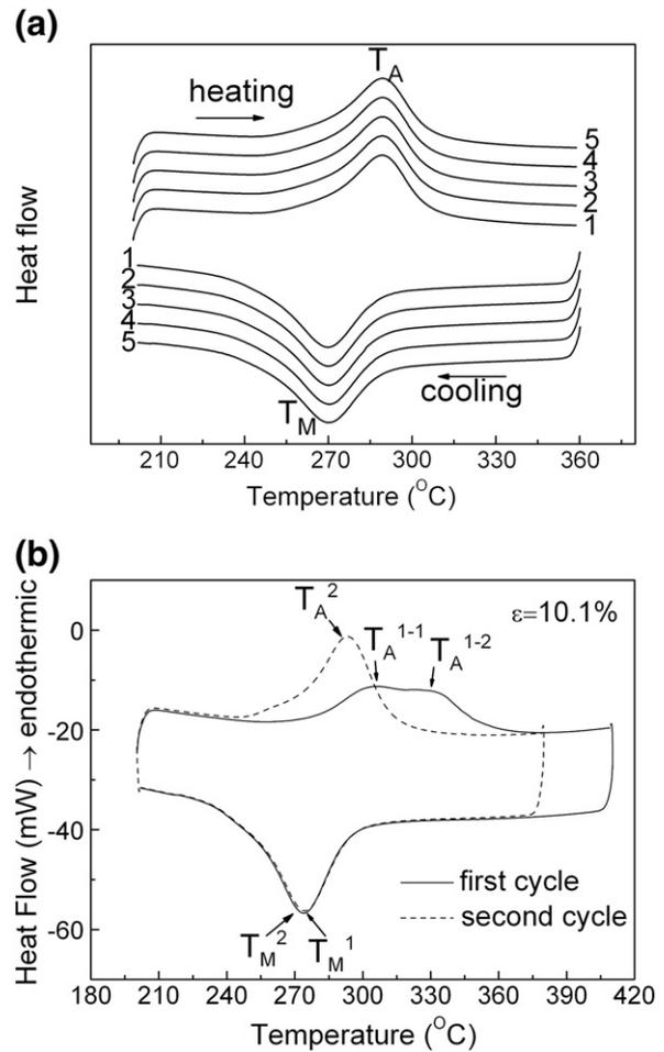
Fig. 2. Transformation behavior of the annealed  $\text{Ni}_{43}\text{Mn}_{43}\text{Co}_7\text{Sn}_7$  alloy after (a) different thermal cycles, the number of thermal cycles is indicated and (b) deformation to 10.1%.
