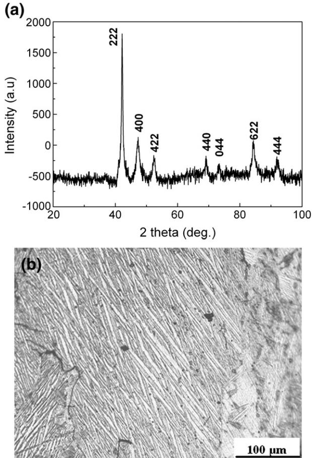
Fig. 1. (a) XRD pattern and (b) optical image of  $\text{Ni}_{43}\text{Mn}_{43}\text{Co}_7\text{Sn}_7$  (at.%) alloy at room temperature.
