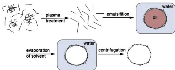
**Scheme 1.** Schematic illustration of the preparation of CNT hollow microspheres by O/W Pickering emulsions.
