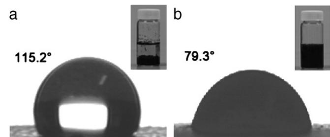
**Fig. 1.** Photographs of the water droplet placed on the surface of the CNT pellet: (a) pristine CNTs and (b)  $O_2$  plasma-treated CNTs (plasma treatment: 20 min). (Insets: photographs of CNT dispersions (0.03 wt.%) in water after staying 48 h from preparation.)
