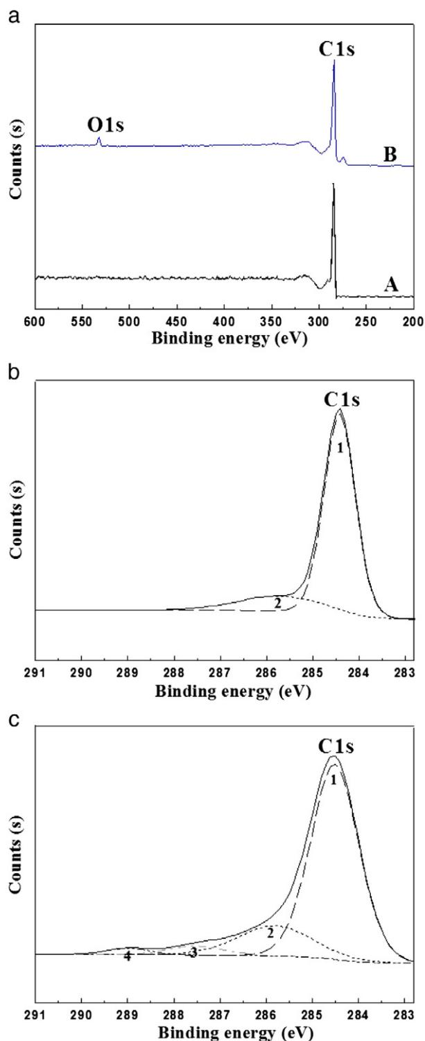
**Fig. 2.** XPS spectra of CNTs. (a) A: pristine CNTs, B:  $O_2$  plasma-treated CNTs, (b) C1s spectra of pristine CNTs, and (c) C1s spectra of  $O_2$  plasma-treated CNTs (plasma treatment time: 20 min).
