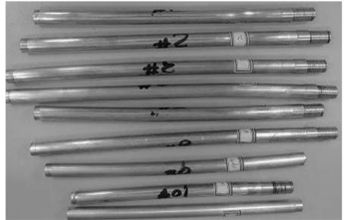
Fig. 2. Top view of hydrostatically extruded bars at room temperature after hot conventional extrusion.
