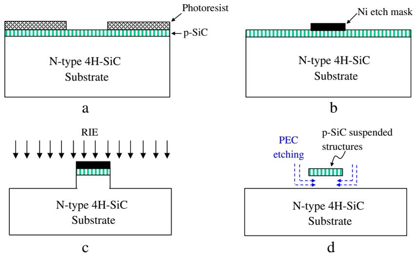
**Fig. 1.** Schematic of the single-crystal SiC MEMS fabrication process: (a) starting material with p-SiC on the n-SiC substrate; (b) photolithography and Ni mask lift-off; (c) RIE etching; and (d) PEC etching with p-SiC MEMS structures released.
