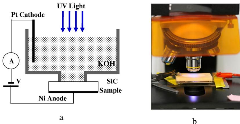
**Fig. 2.** (a) Schematic and (b) micrograph of the PEC etch setup.
