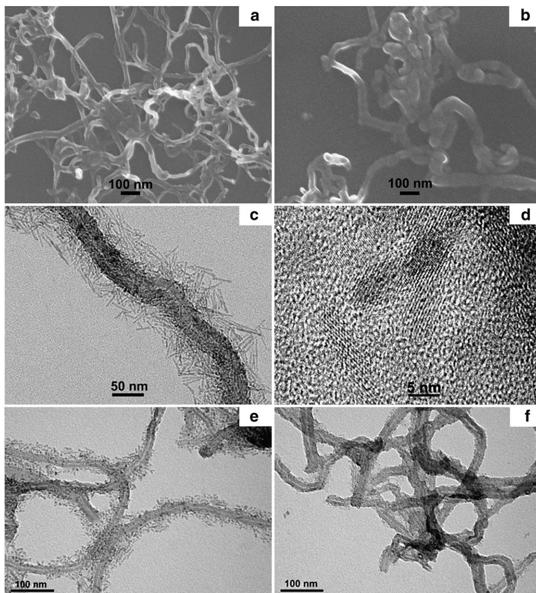
Fig. 1. (a) SEM image of the pristine MWCNTs; (b) SEM, (c) typical TEM and (d) HRTEM images of hybrid-1; (e) TEM image of hybrid-2 and (f) TEM image of hybrid-3.
