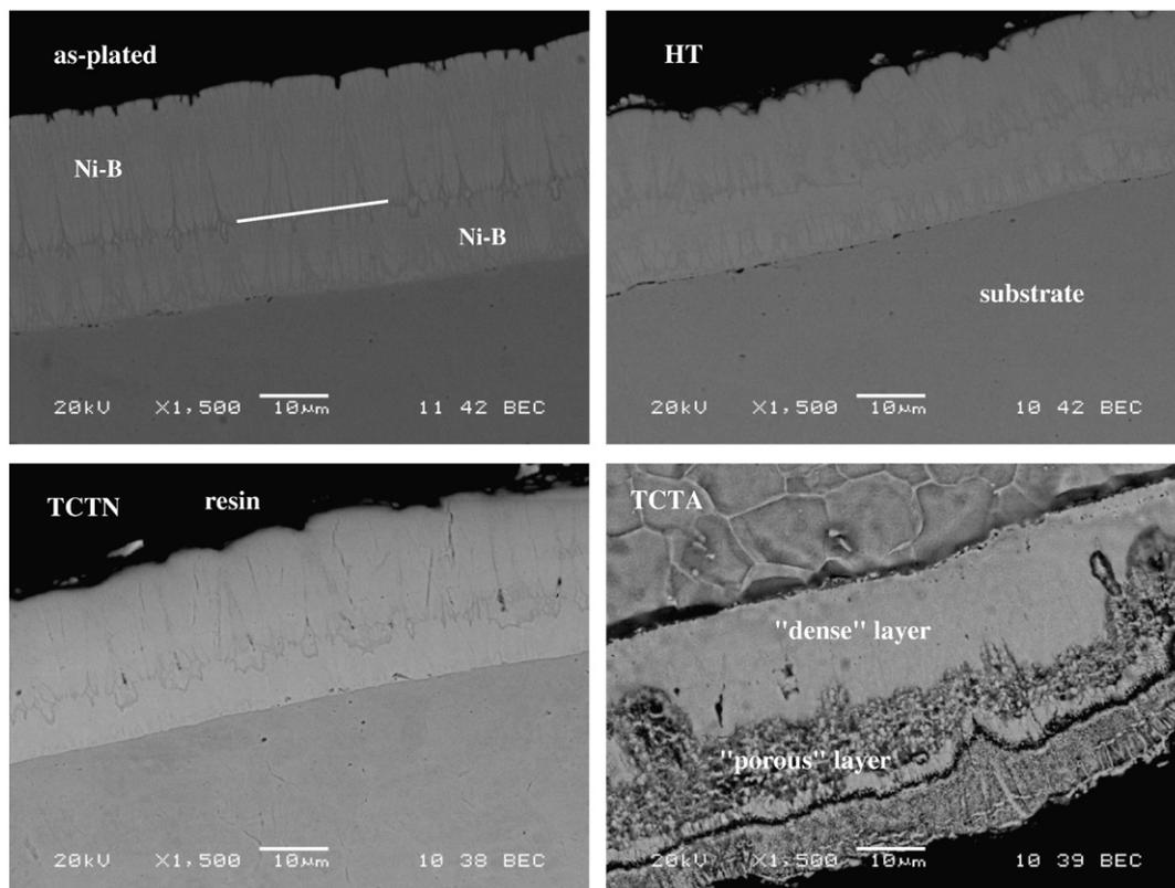
**Fig. 1.** SEM cross section morphology of Ni–B coating with replenishment.
