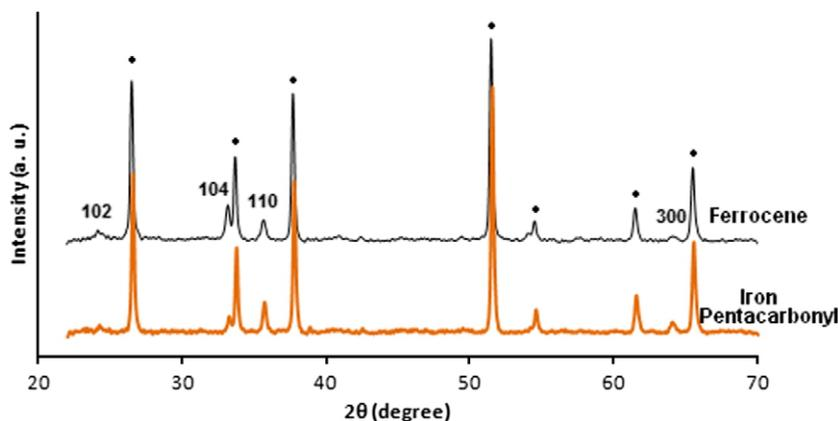
Fig. 1. XRD pattern of the films prepared by ferrocene and iron pentacarbonyl. (102), (104), (110) and (300) reflections correspond to hematite. The peaks labelled with (●) correspond to the  $\text{SnO}_2$  in the FTO substrate.
