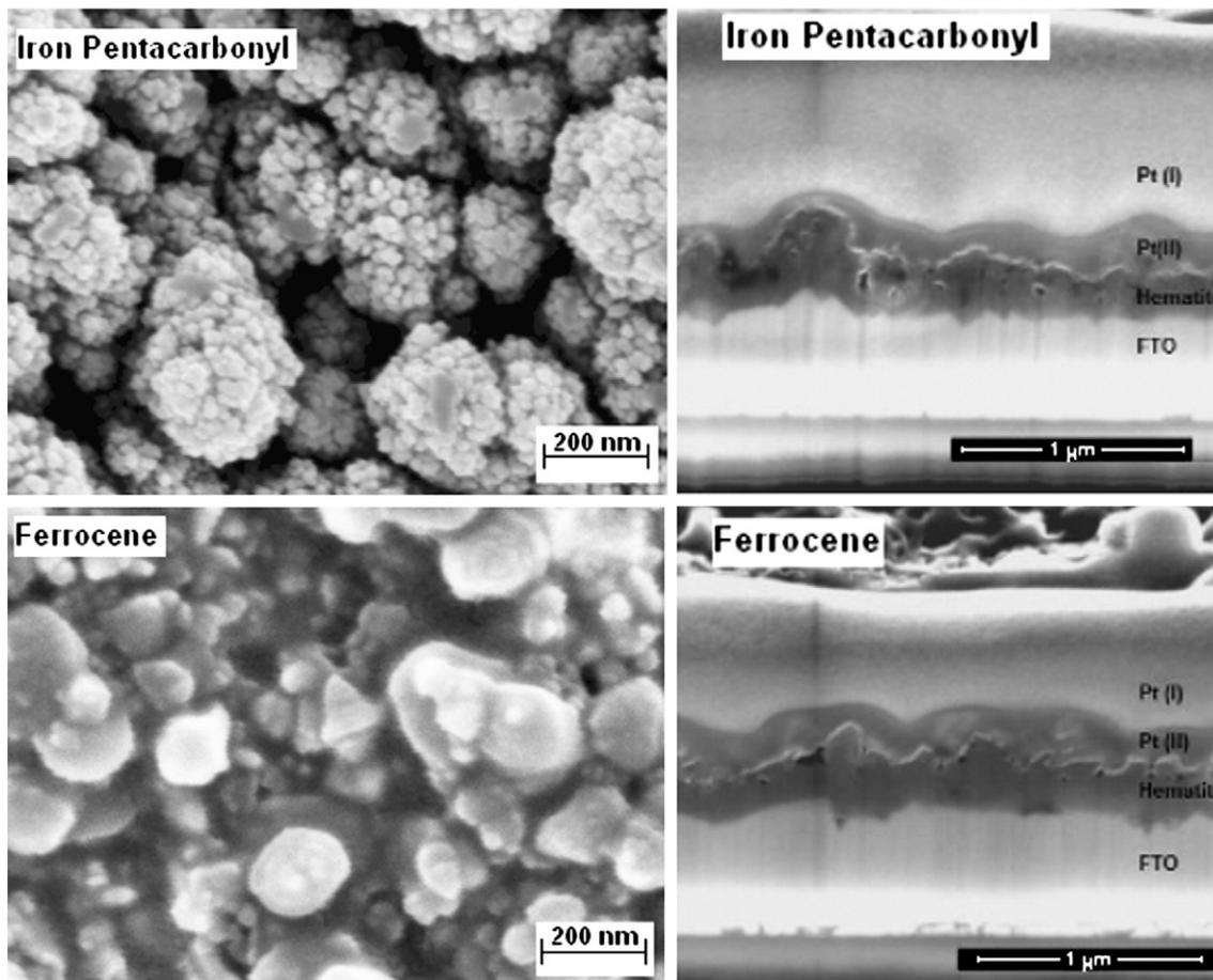
Fig. 2. SEM micrographs of hematite films showing surface morphology and the thickness of the films prepared by iron pentacarbonyl and ferrocene. Pt(I) and Pt(II) are the platinum layers deposited by ion beam and electron beam, respectively. The SEM pictures of the cross section are obtained at a tilt angle of  $52^\circ$ .
