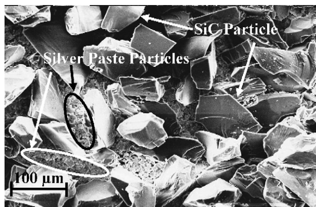
Fig. 1. SEM micrograph (SEI) shows the SiC particles pasted on the surface of Al metal by silver paste.
