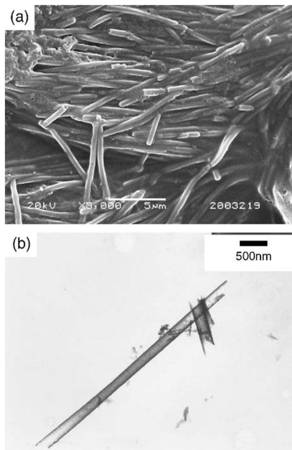
Fig. 2. Morphologies of PANI microtubes. (a) SEM image; (b) TEM image.
