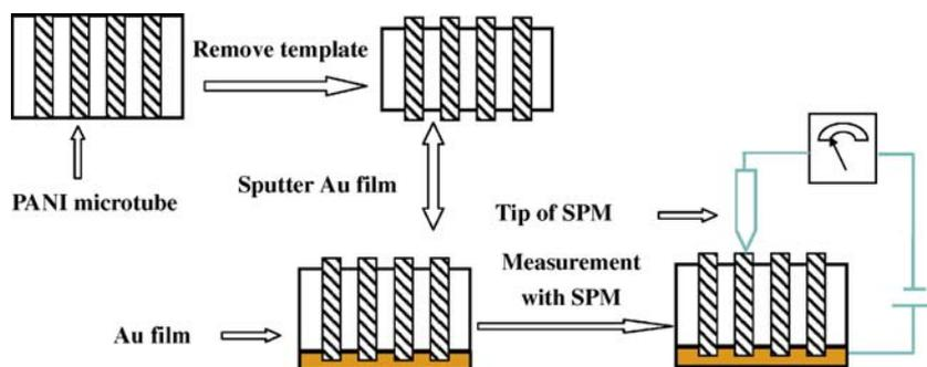
Fig. 1. Schematic process for the measurement of the electrical property of PANI microtube.
