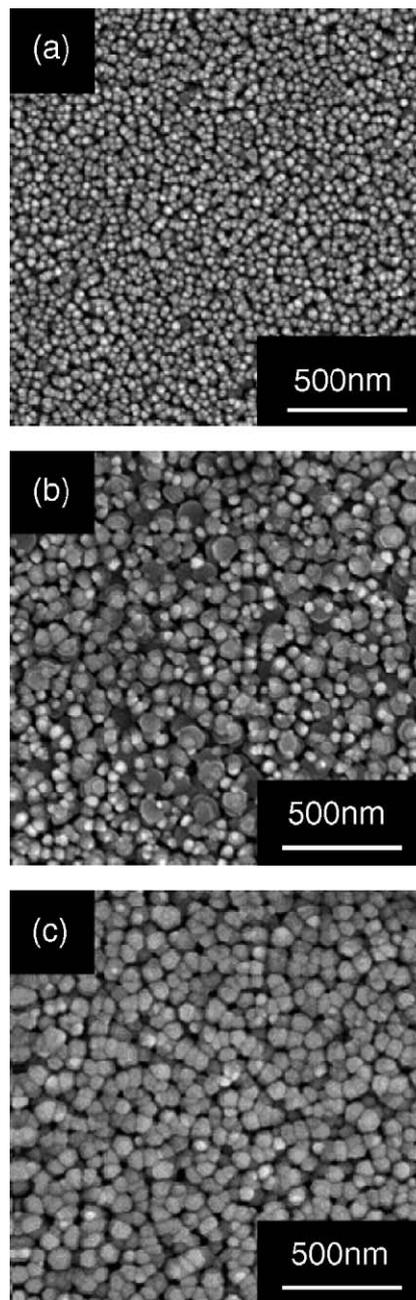
Fig. 1. SEM surface images of the N-doped ZnO thin films grown at different temperatures: (a) 300 °C; (b) 400 °C; (c) 500 °C.
