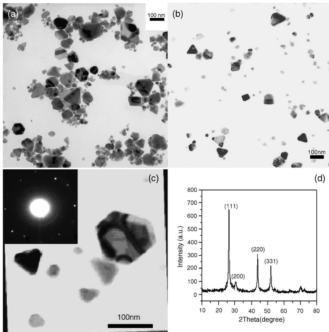
Fig. 1. TEM images of CdS nanoplates prepared in water under different cadmium acetate concentrations (a)  $0.02 \text{ mol}\cdot\text{dm}^{-3}$ ; (b)  $0.05 \text{ mol}\cdot\text{dm}^{-3}$ ; (c) TEM image of a single triangle and hexagonal CdS nanoplates under cadmium acetate  $0.05 \text{ mol}\cdot\text{dm}^{-3}$ . The inset corresponds to the SAED pattern of the CdS nanoplates (d) XRD pattern of the product.
