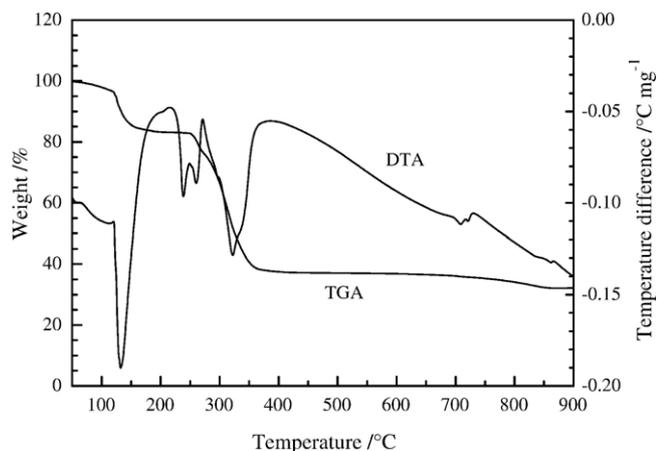
Fig. 1. DTA/TGA curves of the precursor powder prepared by the spray-drying method.
