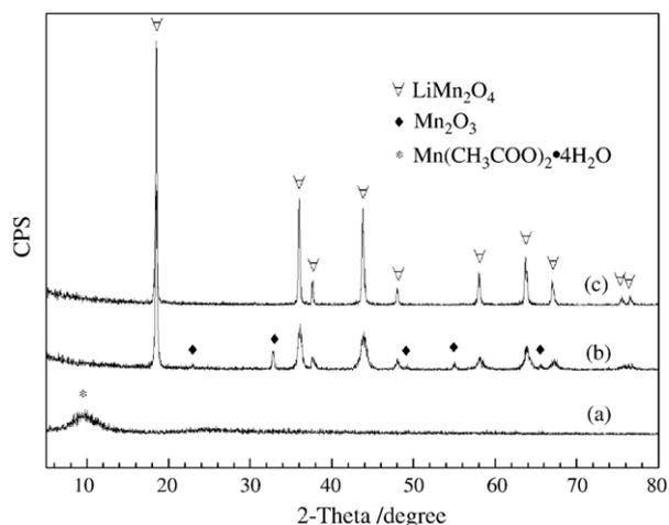
Fig. 2. XRD patterns of the as-prepared powders. a: Precursor; b: after being sintered at 500 °C for 6 h; c: after being sintered at 750 °C for 5 h.
