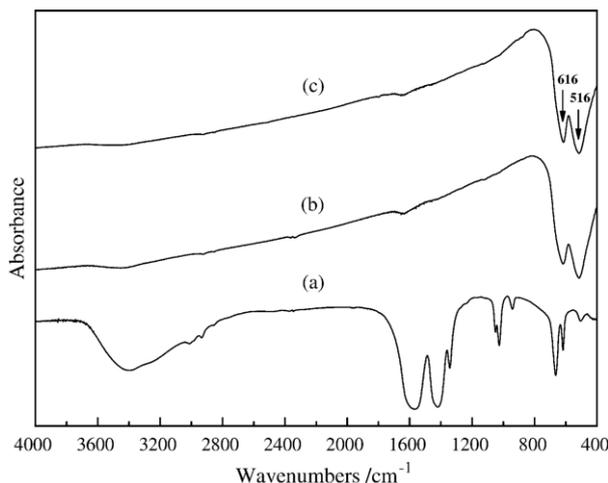
Fig. 3. FTIR spectra of the as-prepared powders. a: Precursor; b: after being sintered at 500 °C for 6 h; c: after being sintered at 750 °C for 5 h.
