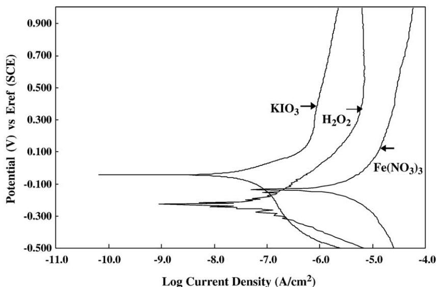
Fig. 1. Potentiodynamic polarization curves of different oxidizers with 5 wt.% contents.
