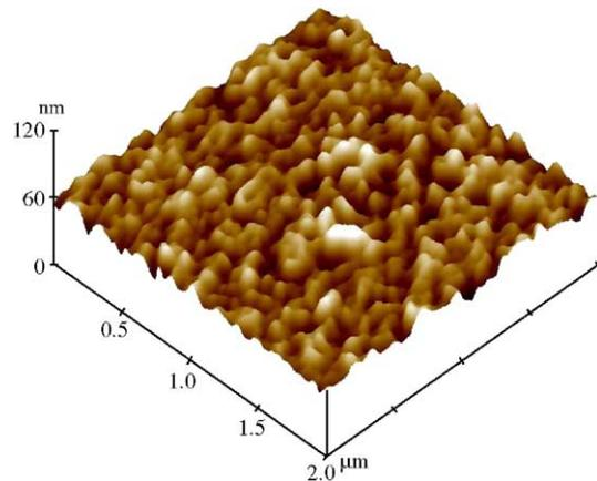
Fig. 2. AFM image of the (Ti,Al)(O,N) film's surface topography (sample 4#).
