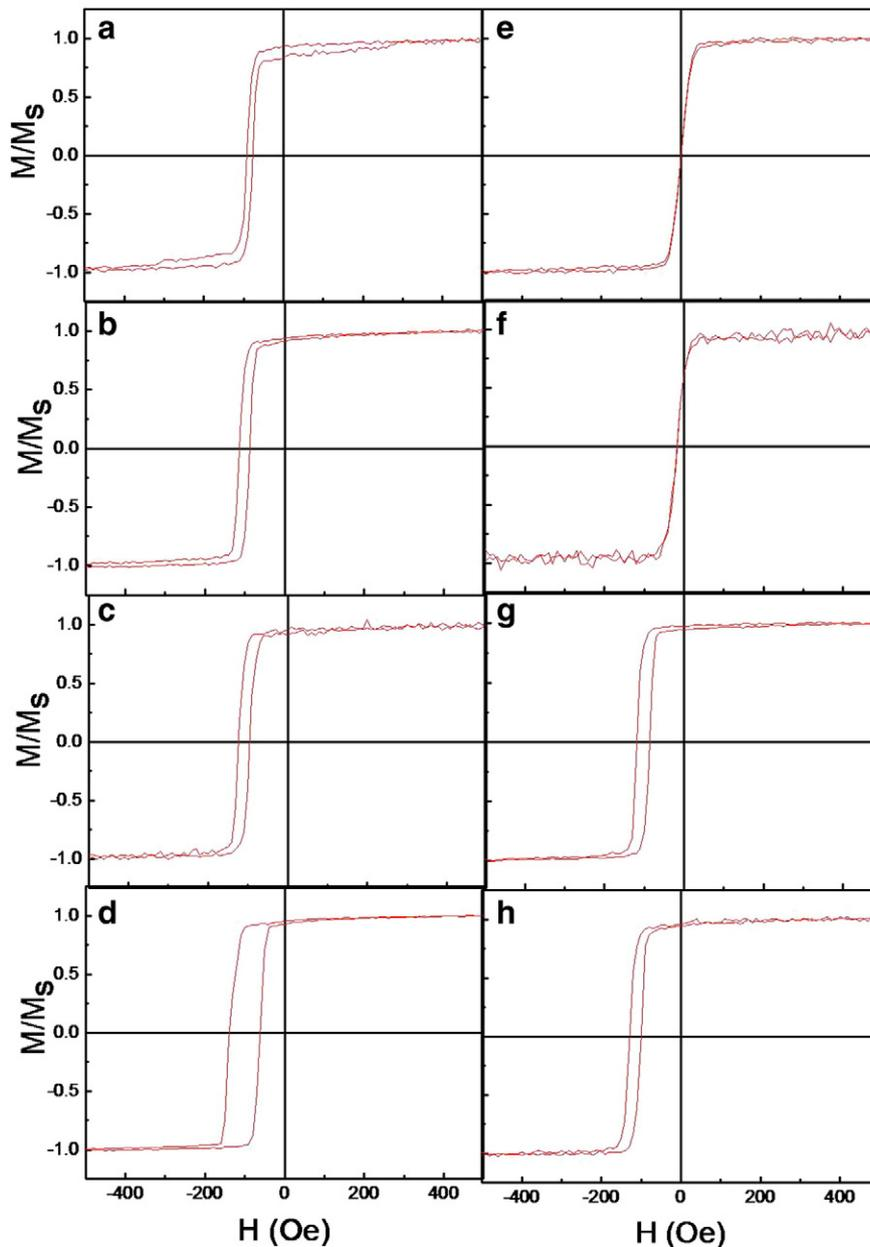
Fig. 1. Magnetic hysteresis loops of FeMn/NiFe films with working pressure of (a) 4 mTorr, (b) 6 mTorr, (c) 8 mTorr, and (d) 10 mTorr, and with Ta thickness of (e) 0 nm, (f) 5 nm, (g) 10 nm, (h) 20 nm.
