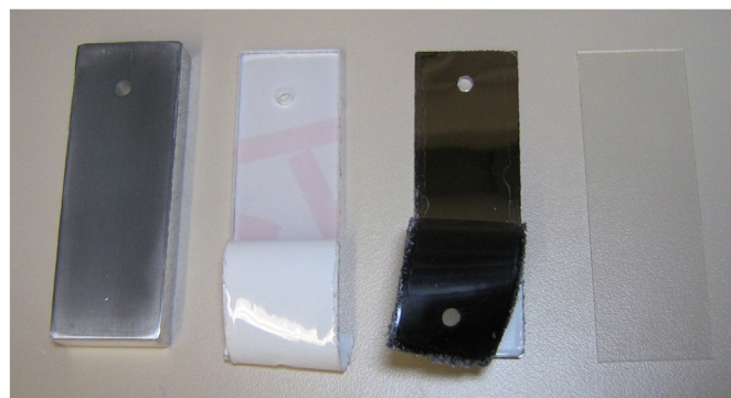
Fig. 1. Samples prepared from each substrate material under study. From left to right: aluminum, polycarbonate, stainless acid-proof steel and glass. Polycarbonate and stainless steel sheets had a protective plastic film which was removed after sample cutting.
