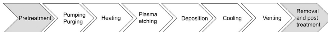
Fig. 1. Sequential steps of deposition processes. In the case of the PVD processes, the steps Pumping, Purging and Venting have been included into the steps Heating and Cooling, respectively. In the case of the CVD process, the step Pumping/Purging was included into the step Heating; the steps Plasma etching and Venting are absent.
