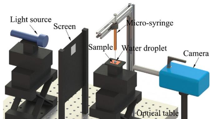
Fig. 2. The contact angle measurement facility.
