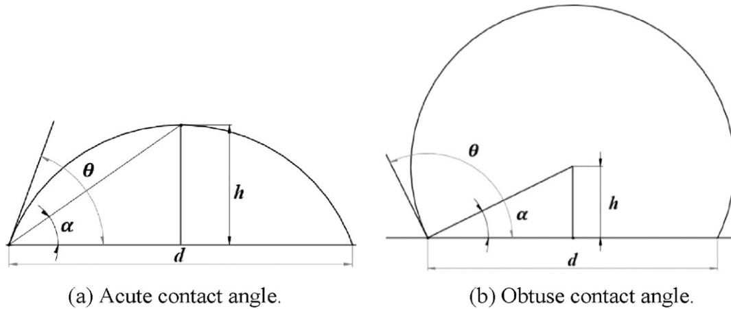
Fig. 1. Schematic drawing of the sessile drop analyzed by the half-angle method.
