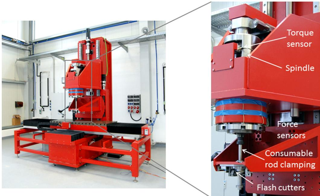
Fig. 2. Friction surfacing equipment.
