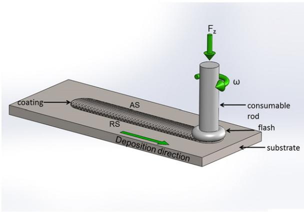
Fig. 1. Schematic description of the friction surfacing process.
