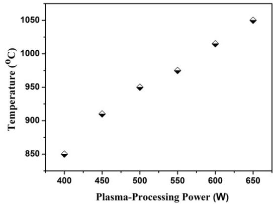
Fig. 2. Sample temperature as a function of RF plasma-processing power.
