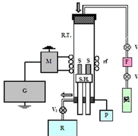
Fig. 1. A schematic of the nitriding system.
