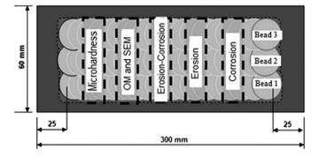
Fig. 1. Scheme details of welded deposits and sample collection.
