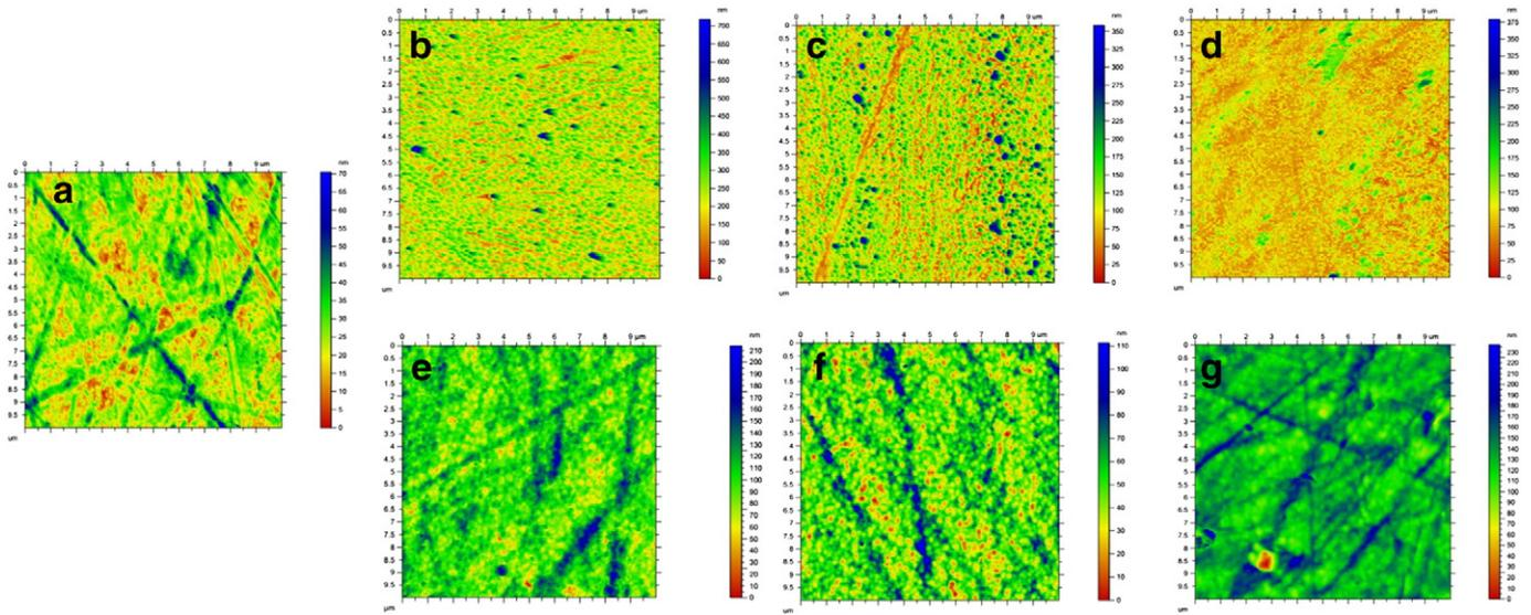
**Fig. 1.** AFM pictures of: a) unmodified substrate, PEEK etched in: b) oxygen plasma, c) nitrogen plasma, d) methane plasma, carbon coating deposited onto PEEK using the preliminary plasma processing in: e) oxygen, f) nitrogen, g) methane.
