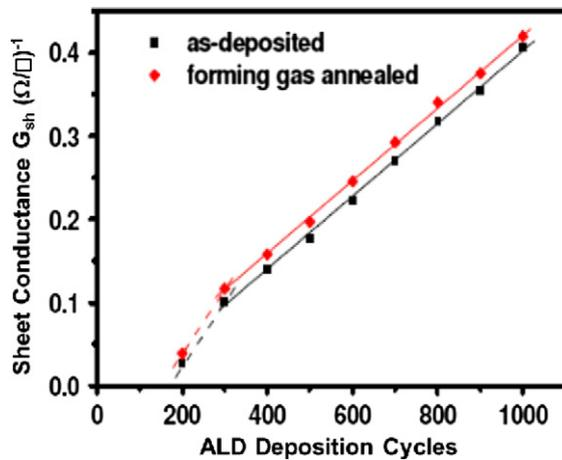
Fig. 2. Electrical measurements of sheet conductance  $G_{sh}$  of Pt films exhibit good linear relationship as a function of the number of ALD deposition cycles.
