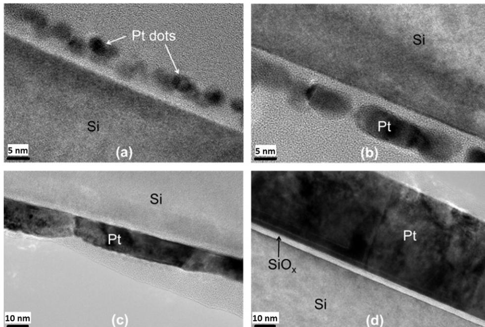
Fig. 3. TEM cross-sections of ALD depositions of Pt at 300 °C for different thickness stage: (a) 50 ALD cycles, (b) 100 ALD cycles, (c) 200 ALD cycles, and (d) 1000 ALD cycles.
