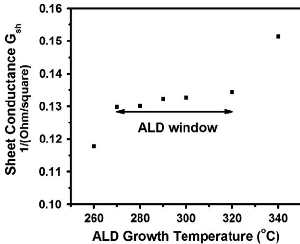
Fig. 1. Sheet conductance of as-deposited Pt film as a function of growth temperature for 400 ALD cycles to establish the process window of stable Pt growth.
