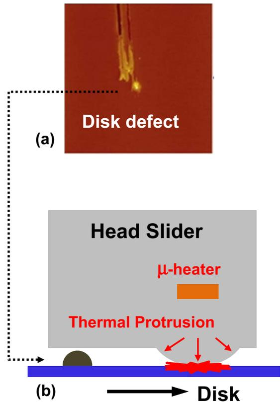
Fig. 1. Two different HDI contact modes. (a) contact with a disk defect; (b) bulk surface contact.
