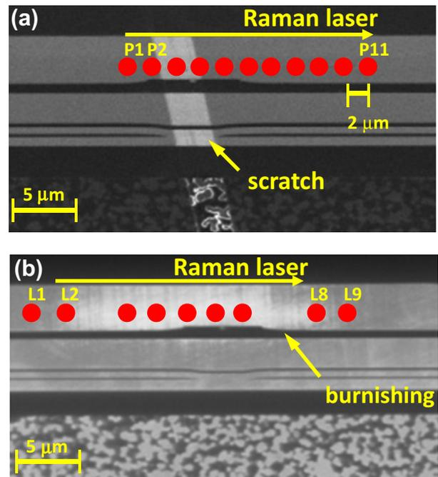
Fig. 2. Micro-Raman measurements on the (a) scratch and (b) burnishing head carbon film.
