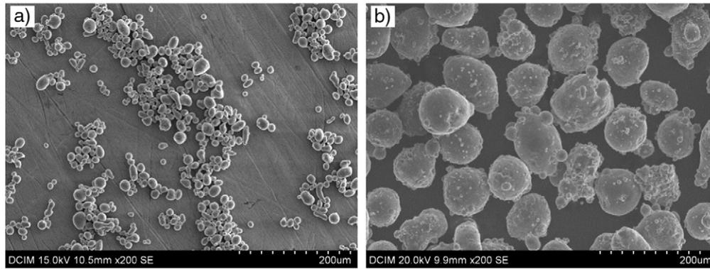
Fig. 1. SEM micrograph of (a) pure Al powders and (b) Al11Si powders.
