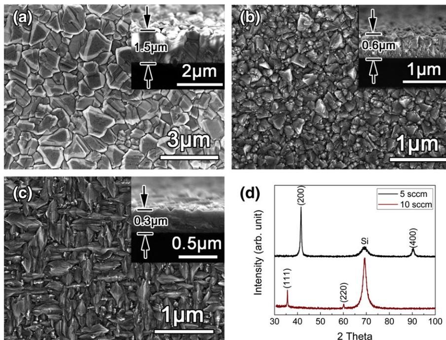
**Fig. 1.** (a–c) SEM surface and cross-sectional images of the pure diamond and pure  $\beta$ -SiC films: (a) pure diamond film deposited at  $\text{CH}_4 = 5.5 \text{ sccm}$ , growth time = 8 h; (b) pure  $\beta$ -SiC film deposited at TMS = 10 sccm, growth time = 6 h; (c) pure  $\beta$ -SiC film deposited at TMS = 5 sccm, growth time = 6 h. (d) XRD patterns of the  $\beta$ -SiC films shown in (b) and (c).
