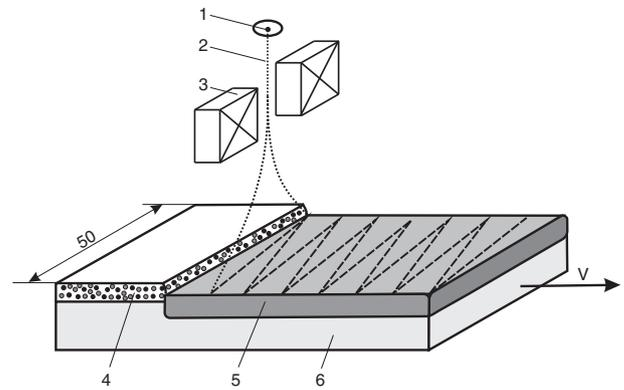
**Fig. 1.** Schematic diagram of non-vacuum electron-beam cladding of steel plate with the iron-graphite powder mixture. 1—Outlet, 2—electron beam, 3—electromagnetic scanning device, 4—powder mixture of graphite, iron, and flux, 5—cladding layer, 6—steel substrate.
