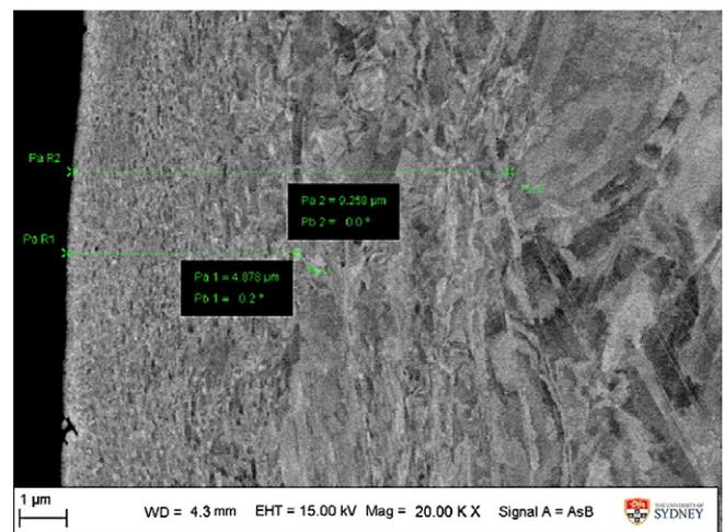
**Fig. 1.** Cross-sectional SEM micrograph of the SMATed sample (SS). The image shows the grain refinement near the surface inside the zone affected by SMAT. The latter extends to beyond 200  $\mu\text{m}$  (outside of the image).
