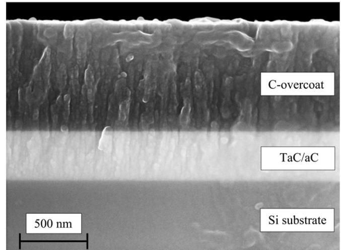
**Fig. 1.** Fracture cross section of the coating with the thickest carbon overcoat ( $800$  nm), deposited on silicon, imaged by HR-SEM. The two layers of the coating are clearly distinguishable.
