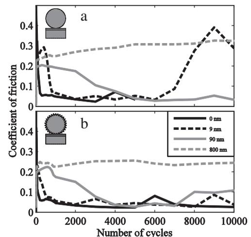
**Fig. 2.** Coefficient of friction as a function of the number of sliding cycles for the coatings deposited on smooth substrates, running against smooth (a) and rough (b) balls.
