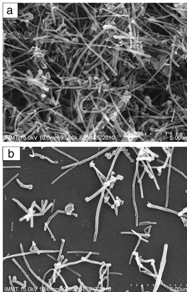
Fig. 1. a. SEM image of as received pristine MWCNT with very large number of cross-linking and entanglement. b. SEM micrograph of well dispersed MWCNT in presence of dispersant GA.
