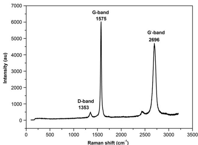
Fig. 2. Raman spectra of multi-walled carbon nanotube.
