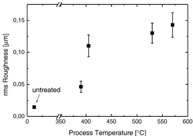
Fig. 1. RMS roughness of CoCr after nitrogen implantation at different process temperatures.
