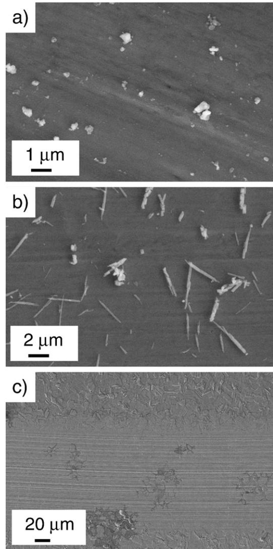
Fig. 2. SEM micrographs of the wear tracks in air of the untreated specimen (a), the specimen nitrided at 390 °C (b) and the wear track in SBF of the specimen nitrided at 570 °C (c).
