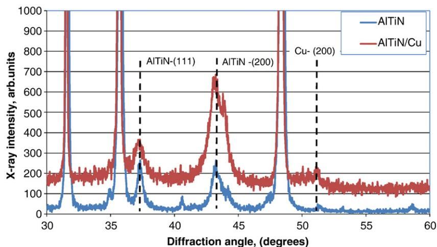
**Fig. 1.** XRD data on AlTiN mono-layered and AlTiN/Cu nano-multilayered PVD coatings.
