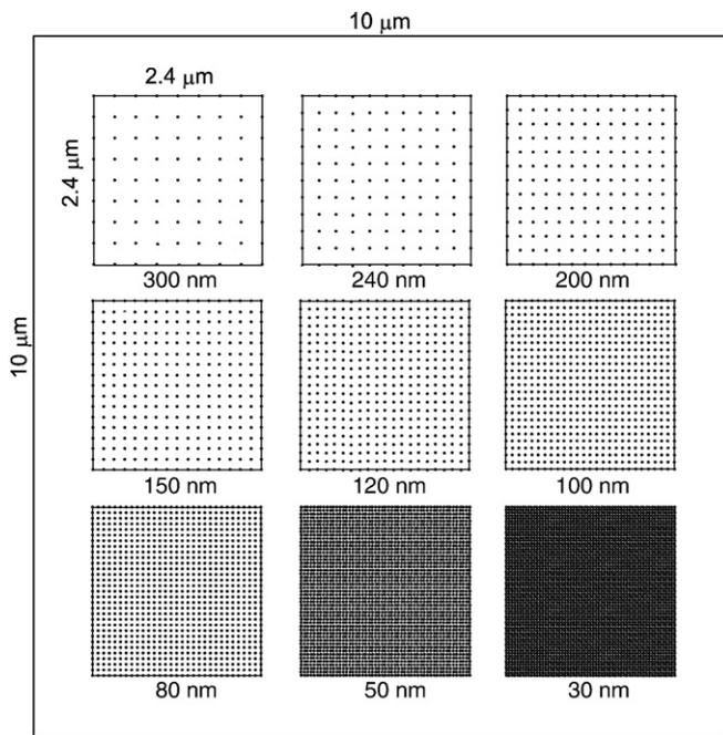
**Fig. 1.** Schematic diagram of the initial pattern fabricated by milling mode of FIB. The initial pattern consists of nine matrices of  $2.4 \mu\text{m} \times 2.4 \mu\text{m}$ , and each matrix is a two-dimensional lattice of implanted dots at a constant interval (30, 50, 80, 100, 120, 150, 180, 240, and 300 nm).
