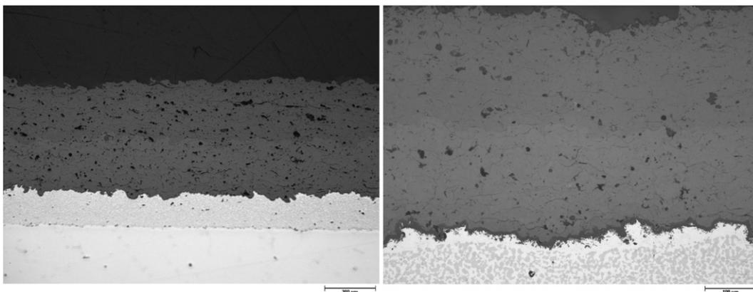
Fig. 2. Micrographs of  $\text{YSZ}/\text{La}_2\text{Hf}_2\text{O}_7$  (left, 1401  $^\circ\text{C}$ , 74 cycles) and  $\text{YSZ}/\text{Gd}_2\text{Zr}_2\text{O}_7$  (right, 1387  $^\circ\text{C}$ , 1782 cycles) coatings after thermal cycling.
