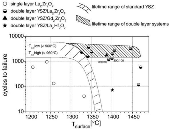
Fig. 1. Cycles to failure for different TBC systems. The numbers 360/40 and 300/100 indicate different layer thickness in micrometer of the double layers (YSZ/pyrochlore).
