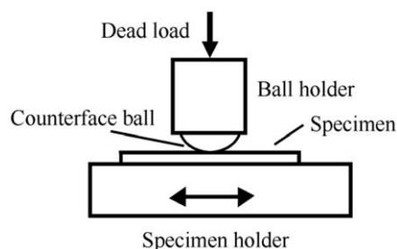
Fig. 1. Contact configuration of the friction pair.
