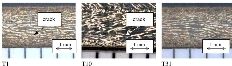
Fig. 1. Superficial photographs of laser nitrided samples. Macro-cracking (T1 and T10) and crack avoidance (T31). Each division: 1 mm.
