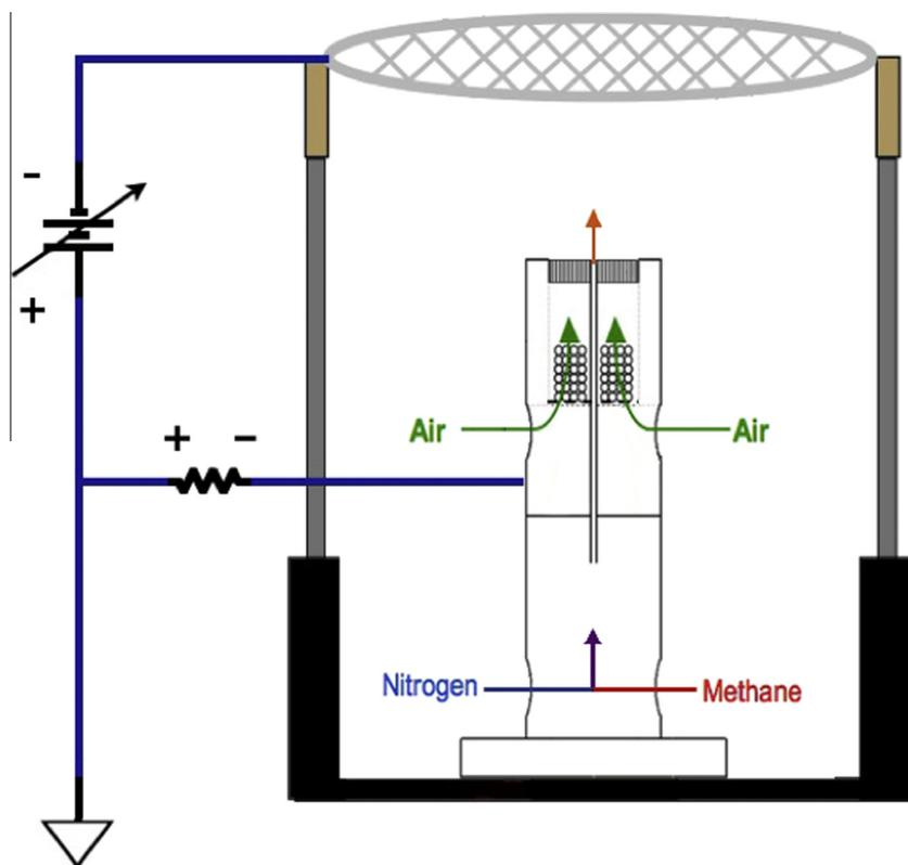
Fig. 1. The above cartoon shows the effective electrical circuit used in ion current measurements and the internal construction of the burner.
