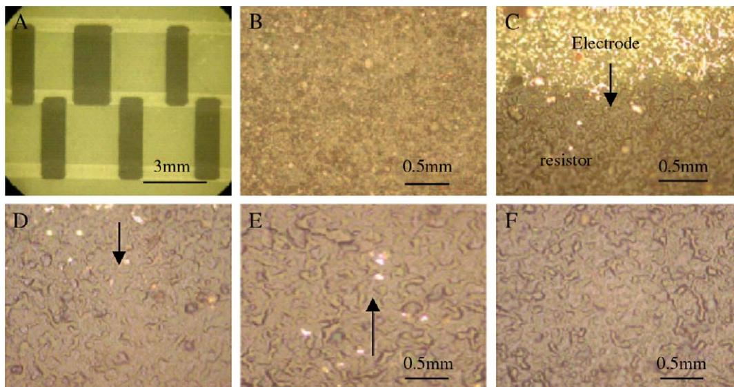
Fig. 1. Morphology and microstructure of resistor and electrode by processing procedure 1. (A) Morphology of interface between resistor and electrode after sintering; (B) microstructure of film after laser irradiation; (C) microstructure of interface between resistor and electrode after sintering; (D), (E), (F) are microstructures of resistor film moving down along resistor long side of (C).
