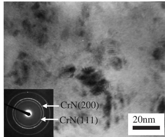
Fig. 1. TEM image and diffraction pattern of the composite CrWN coating.
