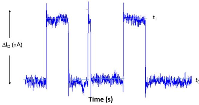
**Fig. 1.** Random telegraph signal in the drain current of a MOSFET and definition of the three relevant parameters: the amplitude  $\Delta I_D$ ; the high (up)  $t_1$  and low (down) time  $t_0$ .
