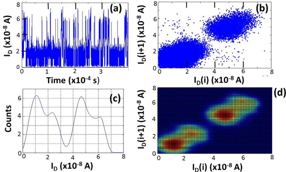
**Fig. 2.** (a) Time series generated by the hidden Markov routine in Matlab and containing a small and a large amplitude RTS; (b) corresponding simple TLP, showing only two clouds of data points; (c) amplitude histogram derived from the time domain signal and (d) colored TLP, showing the presence of the two RTSs.
