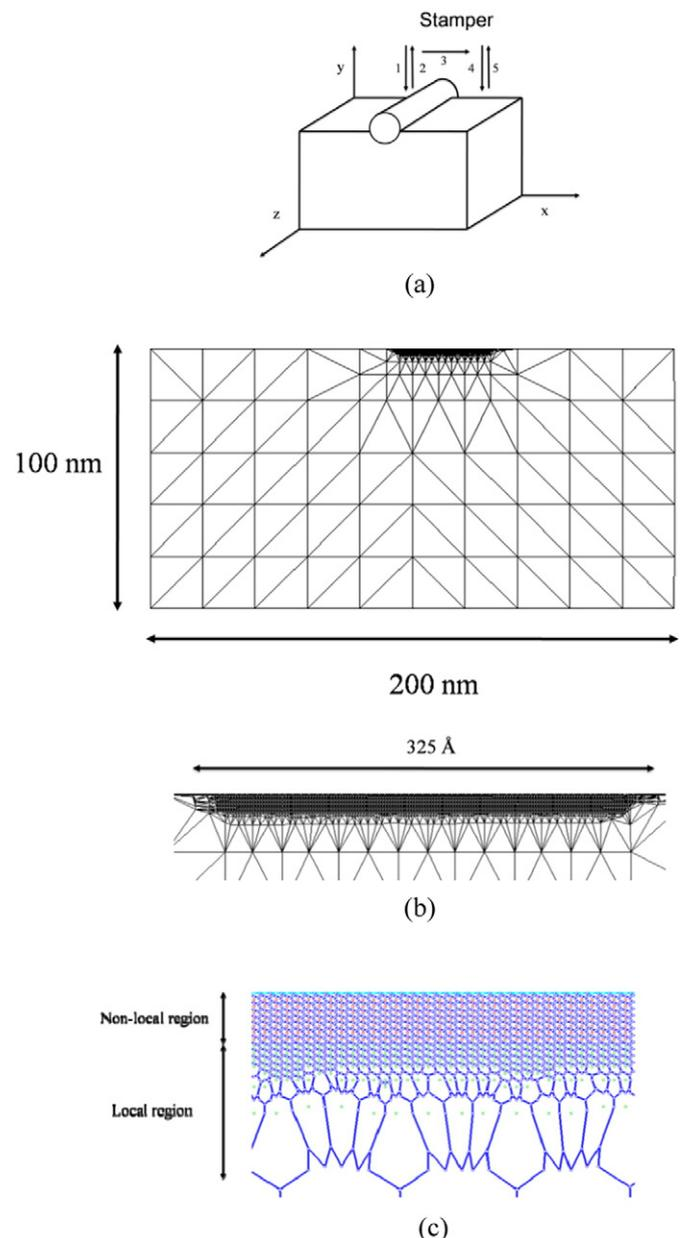
**Fig. 1.** The schematic illustration of nanoimprint on a nanocrystal aluminum thin film.
