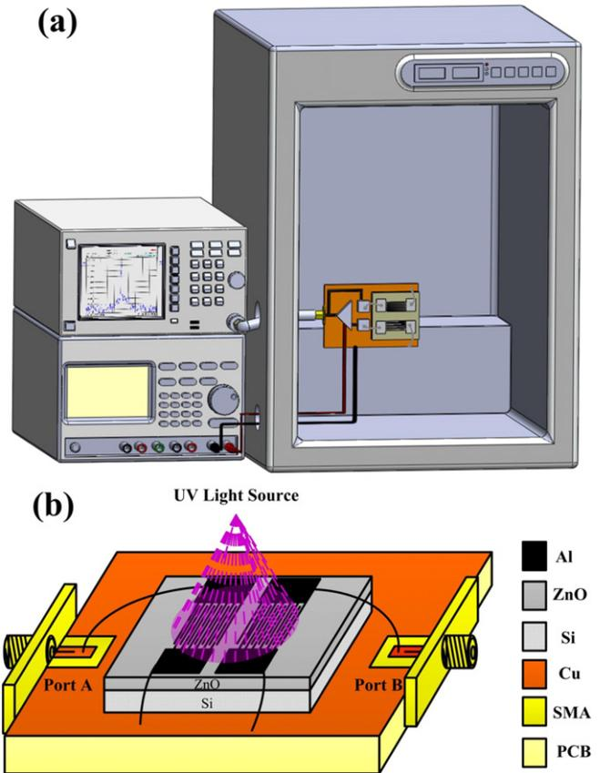
**Fig. 1.** (a) Airtight box system (b) UV light illumination and measurement details.
