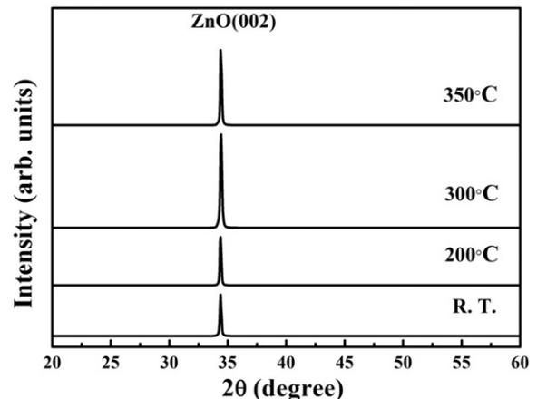
**Fig. 2.** XRD pattern of ZnO thin films deposited with various substrate temperatures.
