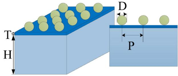
Fig. 1. Schematics of the hybrid Si/PEDOT:PSS cell structure incorporated with Ag nanoparticles on the top surface.
