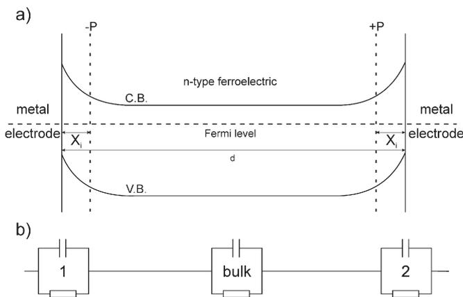
**Fig. 1.** a) Assumed energy band diagram for the  $MFM$  structure showing the two charged sheets in the vicinity of the interfaces and b) equivalent circuit used to characterize the  $MFM$  structure.
