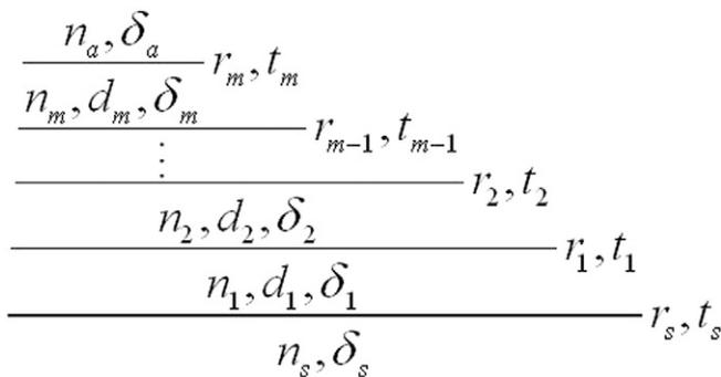
Fig. 1. Schematic representation of  $m$ -layer structure with amplitude reflection and transmission coefficients  $r_m$  and  $t_m$ , ambient environment and substrate refractive indexes  $n_a$  and  $n_s$ , layer thickness  $d_m$ , and optical admittance  $\delta_m$ .
