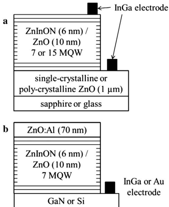
Fig. 1. Schematics of (a) ZnInON/ZnO MQWs structure, (b) solar cells with ZnInON/ZnO MQWs in the intrinsic layer of p-i-n structure.
