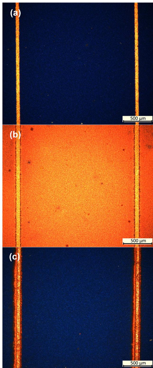
Fig. 1. OM Images of the HIT cell surface: (a) before the electroless plating; (b) after the electroless plating using Cu–EDTA solution; (c) after the electroless plating using Cu–THPED solution.
